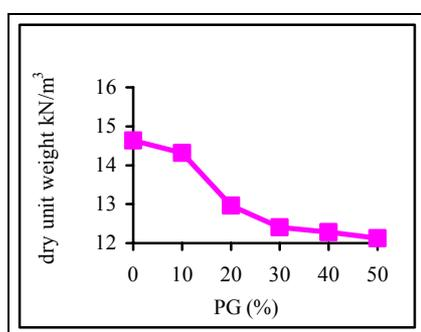
Figure 5. Dry Unit Weight of FaL-G Binders.
