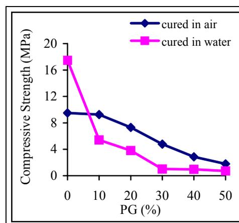
Figure 1. Compressive Strength of FaL-G Binders at 28-days.
