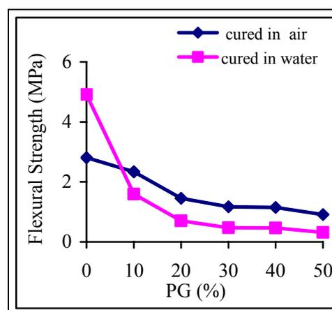
Figure 2. Flexural Strength of FaL-G Binders at 28-days.
