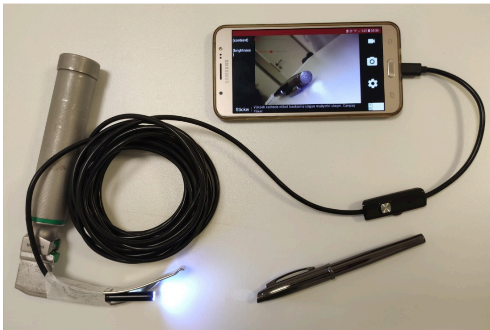
FIGURE 2. The set-up of USB endoscope laryngoscope.
