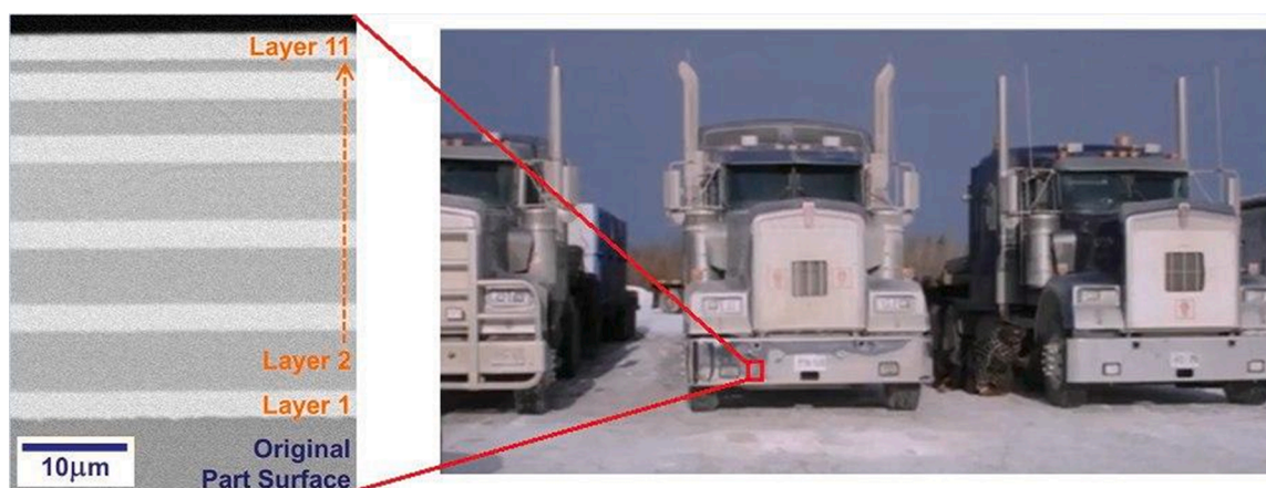
Fig. 41. Haulage truck bumpers coated with a Ni-W multilayer coating, which are claimed to have double the lifetime of conventional hard chromium coatings.
