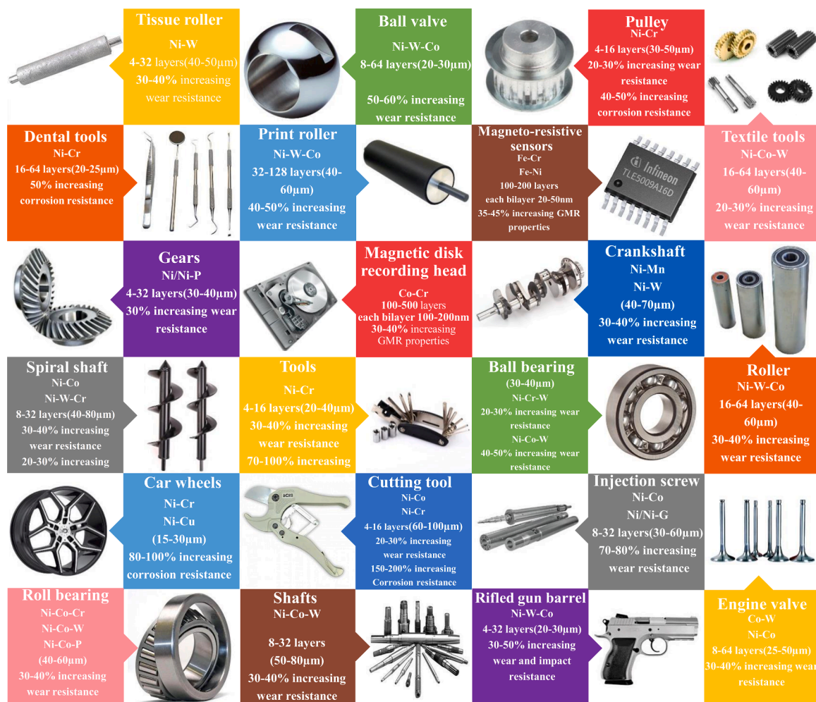
Fig. 42. Potential applications of multilayer electrodeposited coatings for various industrial components, indicating the number of layers, their thickness and improved properties compared to monolithic layers.
