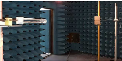
Figure 6. A photograph inside an anechoic chamber during measurements
