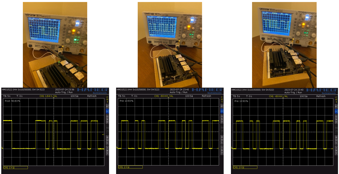
Figure 4. Oscilloscope images obtained using the Nvidia Jetson Nano development board to demonstrate the applicability of random numbers generated through the x \oplus y operation.
