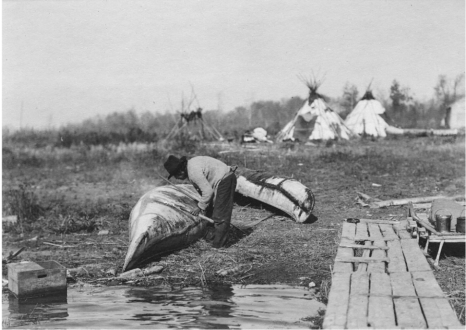
FIGURE 5. Chief Powassin Mending Canoe, c1912. Note burning stick being used to apply balsam fir pitch to seal seams where birch bark sheets stitched together. Result is illustrated in canoe not being worked on where the black bands created by application of pitch are visible. Photograph by Carl Gustav Linde. From the collection of the Lake of the Woods Museum (used by permission).
