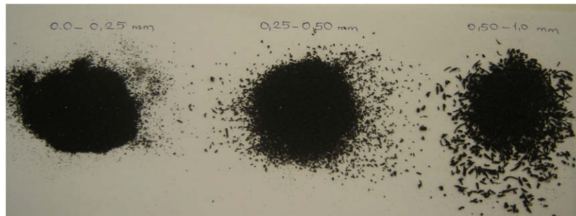
Fig. 1. Rubber waste particles used in the experimental study.
